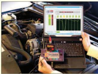
can be determined, with accuracy to within three crankshaft degrees. If the cylinder pressure test indicates a mechanical problem, the EmissFire Detector checks the cylinder in three states—cranking, idle and snap throttle—to identify valve spring, piston ring, intake valve, exhaust valve and valve guide problems.
